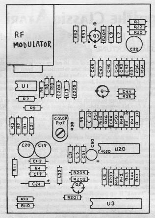
Figure 3. 130XE parts placement diagram.
