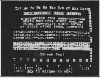
Figure 2A. Composite video output of stock 800XL: worst case grain, blur and smear.
