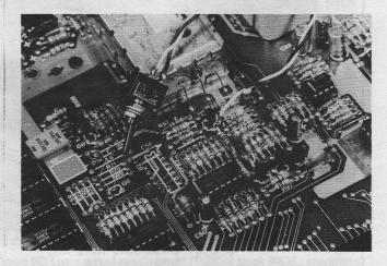
Figure 6. 800XL motherboard after Super Video modification. Note CV Disable switch, empty space for C56, doubled resistors, tantalum capacitor.
