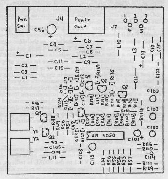
Figure 8. Parts placement for the 600XL
